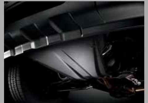
Rugged steel skid plates provide heavy-duty protection for vital underpinnings. Three skid plates (front, mid and aft) are standard on SPORT 4x4s; optional on XLT 4x4s. Mid and aft skid plates are optional on XLT 4x4s. A front plate (shown) is standard on SuperCab 4x2s.
